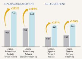
Slip resistance test according to EN ISO 20344:2021, conducted by Intertek Testing Services Shenzhen Ltd., in August 2022; on a scale of 0.0 (without slip resistance) to 1.0 (very high level of slip resistance, e. g. on dry carpeted floors). All SFC shoes are fitted with the patented, slip-resistant Shoes For Crews outsole Tested product: Carrig Low 62201.
